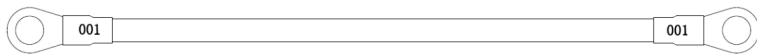
Figure 6-3 Schematic diagram of the series DC cable (picture is for reference only)
