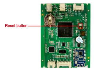
Please note:After restoring the charger to factory setting, you'll need to reset the charger ID and server url, otherwise the charger won't be connected to the back-office server.
