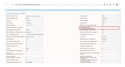
c. Check if off-peak charging is set and if charger's time is correct.
