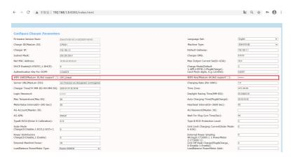
If you check the WiFi setting on the APP, please turn off and back on the charger and connect your mobile to the WiFi emitted by the charger for checking and setting.
