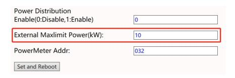
(5) If you choose the PowerMeter.Plesae choise PowerMeter Type, change PowerMeter Addr to the address shown on the meter.
