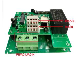
1. Terminal block for CT/meter wiring. The terminal definition is:
