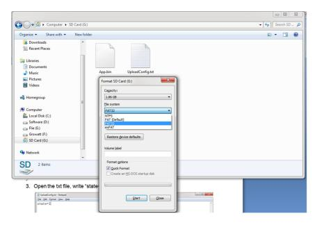
2. In the root directory of the SD card, rename the firmware file as "App.bin". And create a txt file with name of "UploadConfig.txt".
