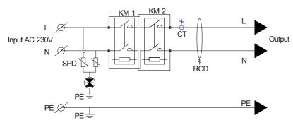
Fig11-1. Main circuit diagram
