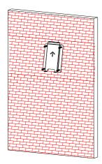
3.1.3 Put the charge point onto the bracket, and fix it with the 2 screws at the bottom of the charge point. The installation is done.
