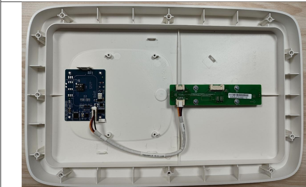
Overall view of the Top cover. Alternative construction. Bottom case are same. Models: NOVO EVA-07S-PU, NOVO EVA-09S-PU, NOVO EVA-12S-PU, are similar to Models: THOR 07AS-P US, THOR 09AS-P US, THOR 12AS-P US, except in different shape of Top cover.
