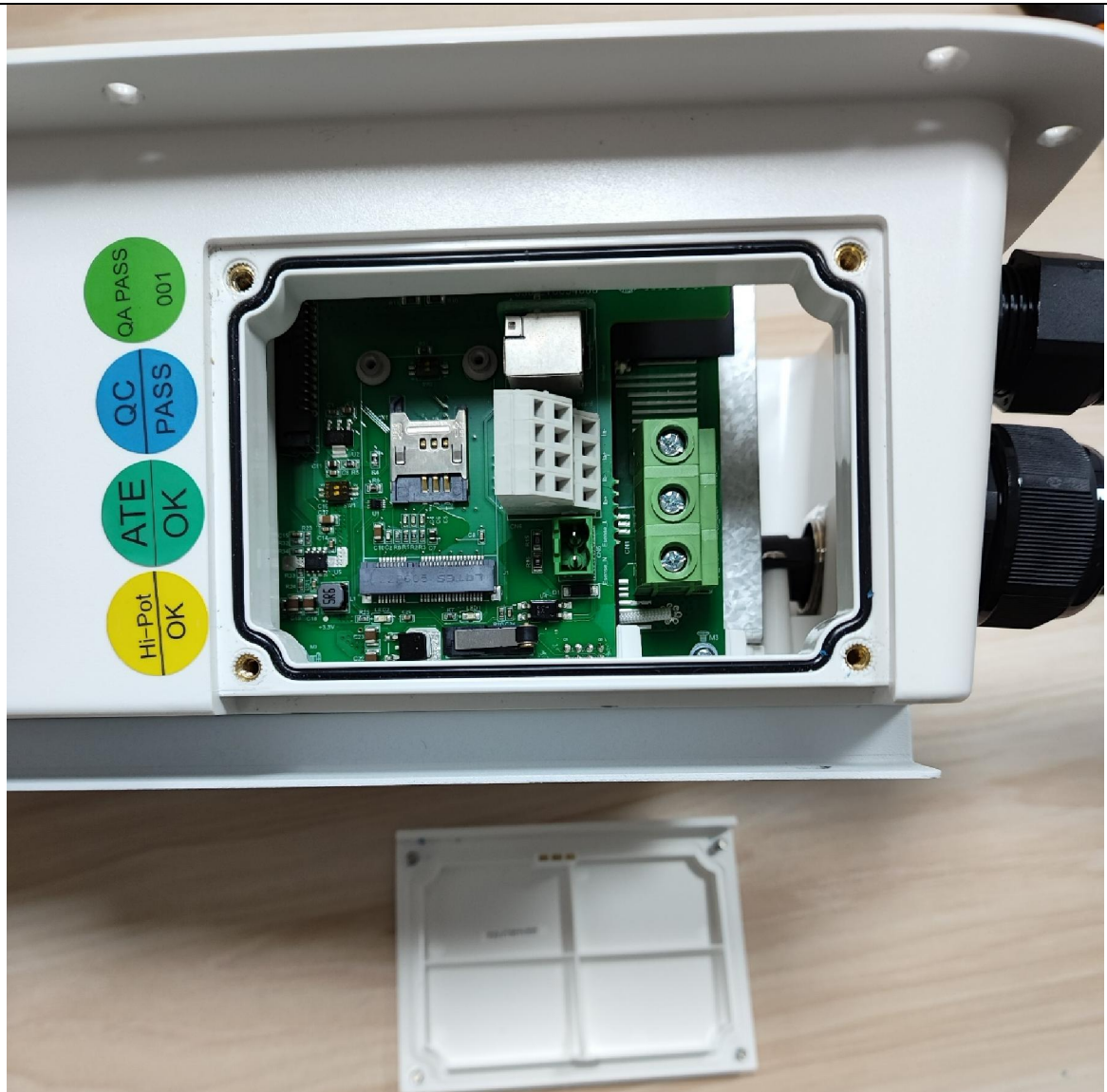
Wiring compartment's protective cover removed
