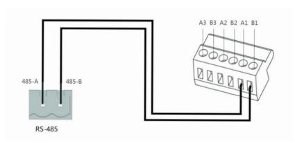
The functions of the A1B1, A2B2, and A3B3 channels are the same.
