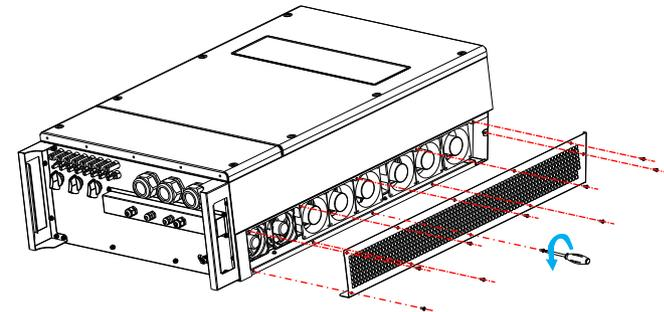
3. Disconnect the fan connector and remove the fan as shown below
