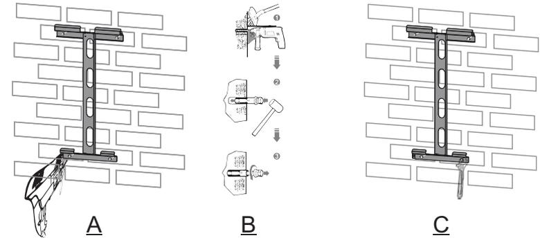
Figure 4-5-1-2 bracket installation
