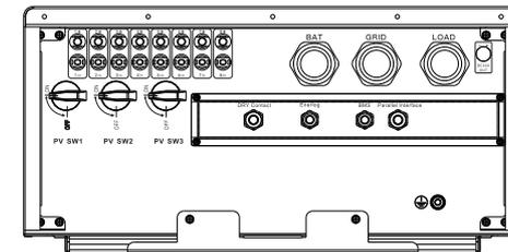
Figure 3-4-1-3 Inverter cable inlet and outlet
