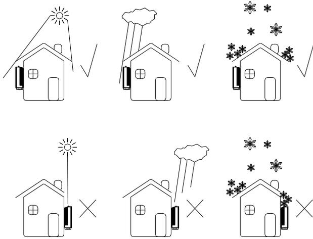
To avoid inverter life span decrease, it is recommended to install shading shield on top of inverter, distance between inverter and top shield please refer to below figure:
