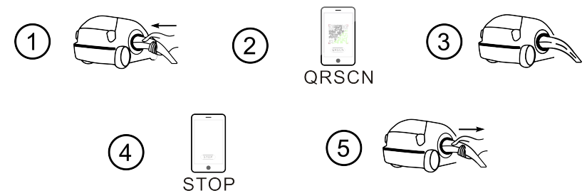
APP/RFID mode operation process flow
