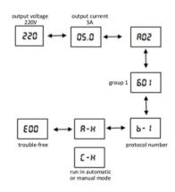
Figure 6 Key operation schematic
