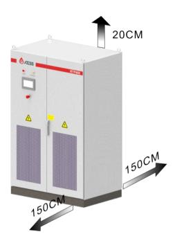
The front of the RTF installation position should provide a clearance of more than 1.5m, while the back and top should have clearances exceeding 1.5m and 0.2m respectively, in order to facilitate installation, efficient heat dissipation, and convenient maintenance.
