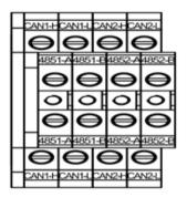
4851-A/B: Connect to the ATESS monitoring system and connect to Enerlog.
