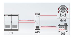
3. There are three circuit breakers inside the ATS, one is the BYPASS switch, and the other two are the GRID switch and the GEN switch. Pay attention to the cabinet label, do not connect to the wrong position, and pay attention to the three-phase phase sequence. Otherwise, the system cannot run normally.
